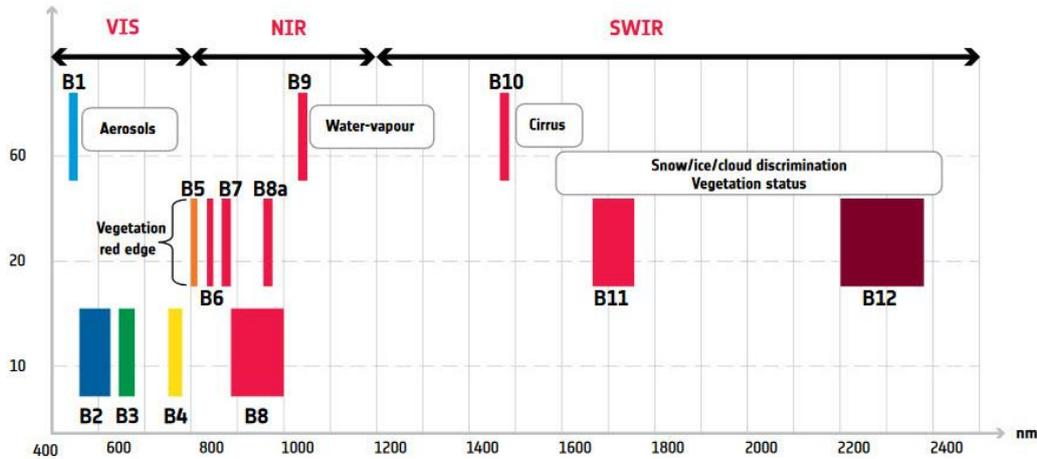
Figure 5. Spatial resolution versus wavelength of the Multi-Spectral Instrument (MSI) onboard Sentinel-2 (source: ESA).
